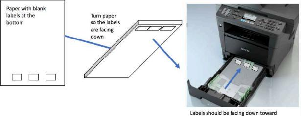
Labels should be facing down toward the bottom of the printer (dashes indicate labels are on the other side of the paper)
